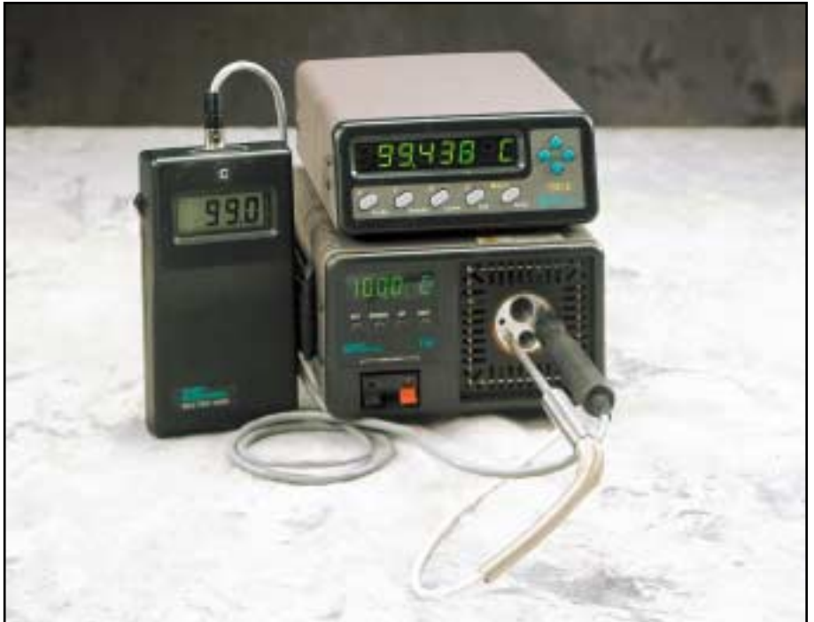
Tweeners are perfect for precision thermometry and as reference thermometers in temperature calibrations (shown here). With LogWare software, they can also now be used for real-time data acquisition.
